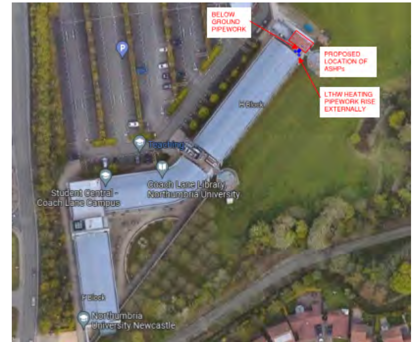
Fig 8: ASHP Location – Blocks F, G, H
