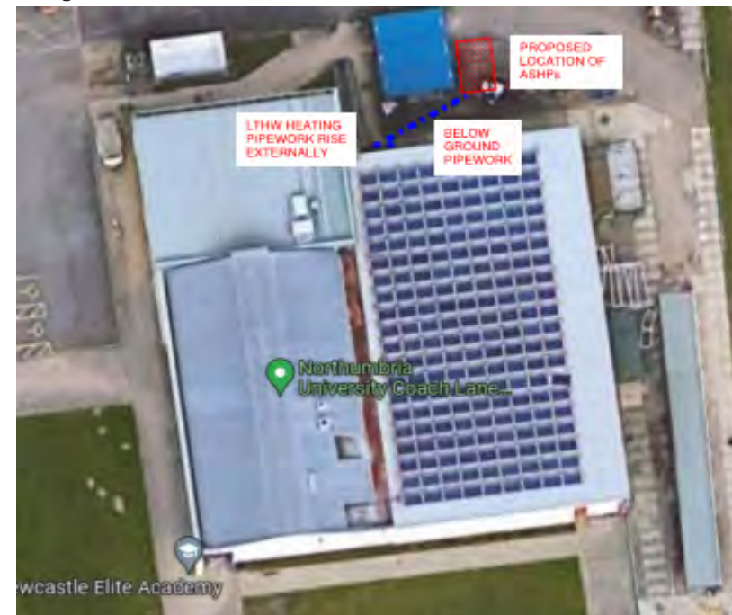
Fig 12: ASHP Location – Sports Hall
