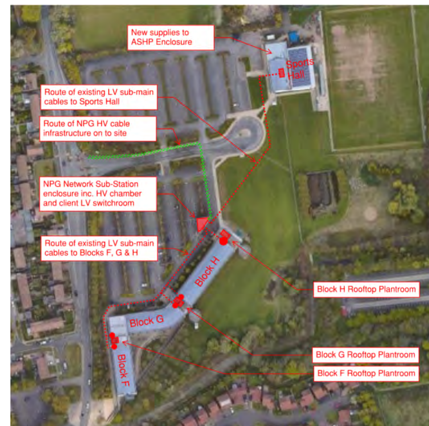
Fig 7: Existing Sitewide Electrical Distribution
