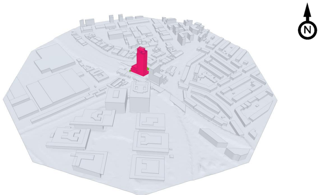
Figure 25 – Proposed Development with Existing Surrounding Buildings, Existing and Proposed Landscaping 3D model used for Computational Fluid Dynamic simulations (view from the south)
