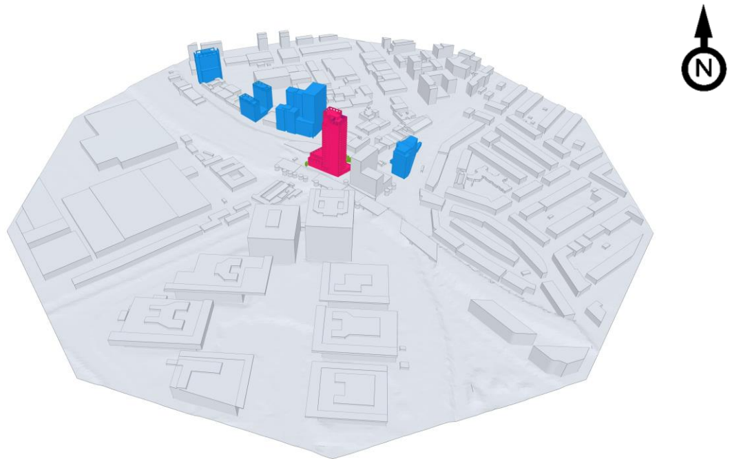
Figure 26 – Proposed Development with Cumulative Surrounding Buildings, Existing and Proposed Landscaping 3D model used for Computational Fluid Dynamic simulations (view from the south)
