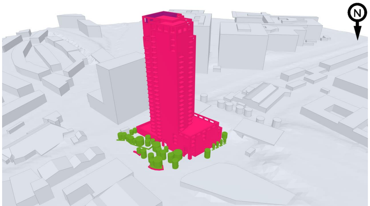
Figure 29 – Proposed Development with Existing Surrounding Buildings, Existing and Proposed Landscaping 3D model used for Computational Fluid Dynamic simulations (view from the north)
