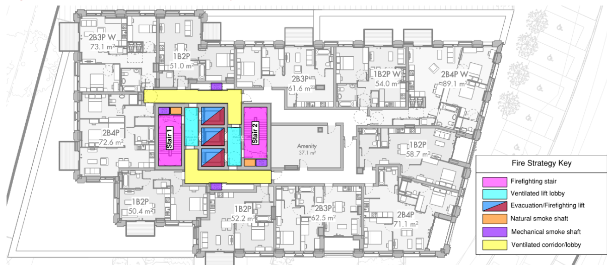
Figure 20 - Horizontal means of escape - 3 rd Floor
