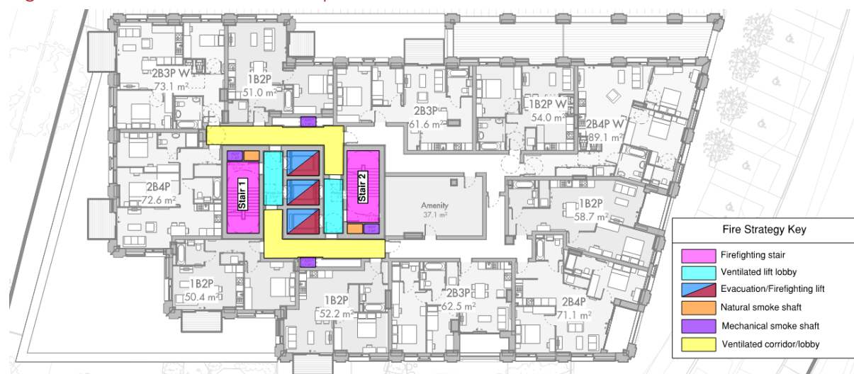
Figure 21 - Horizontal means of escape - 2 nd Floor
