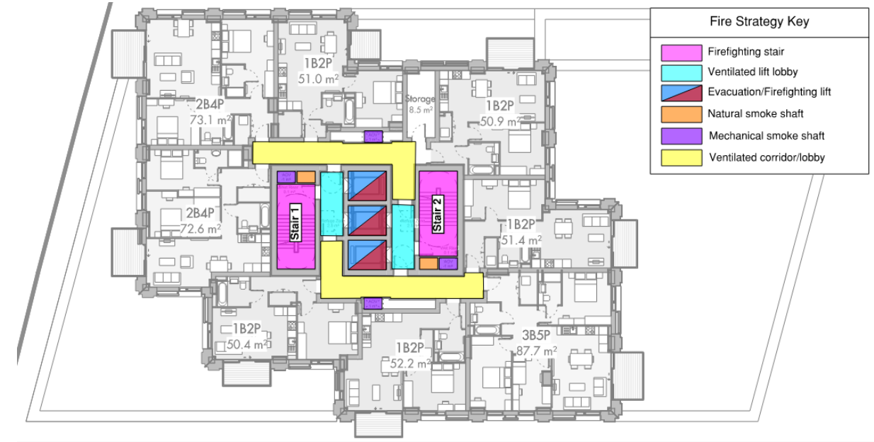
Figure 17 - Horizontal means of escape - 12 th Floor
