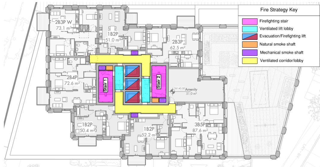
Figure 19 - Horizontal means of escape - 4 th Floor
