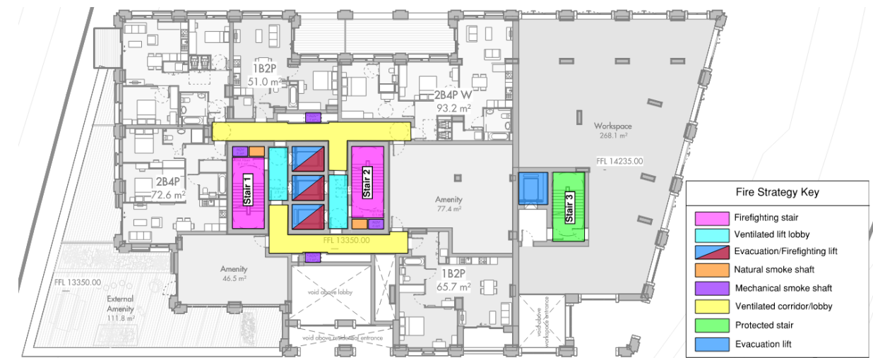
Figure 23 - Horizontal means of escape - Mezzanine Floor
