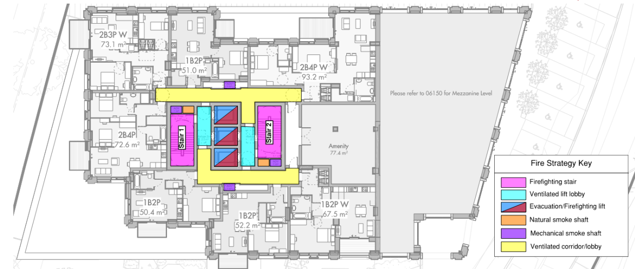
Figure 22 - Horizontal means of escape - 1 st Floor
