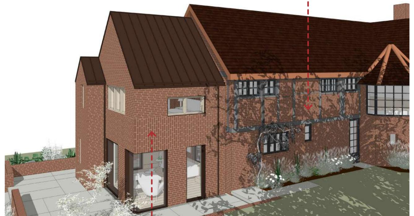
Fig.26: Brick 'panels' proposed to reference the existing post and beam brick infills
