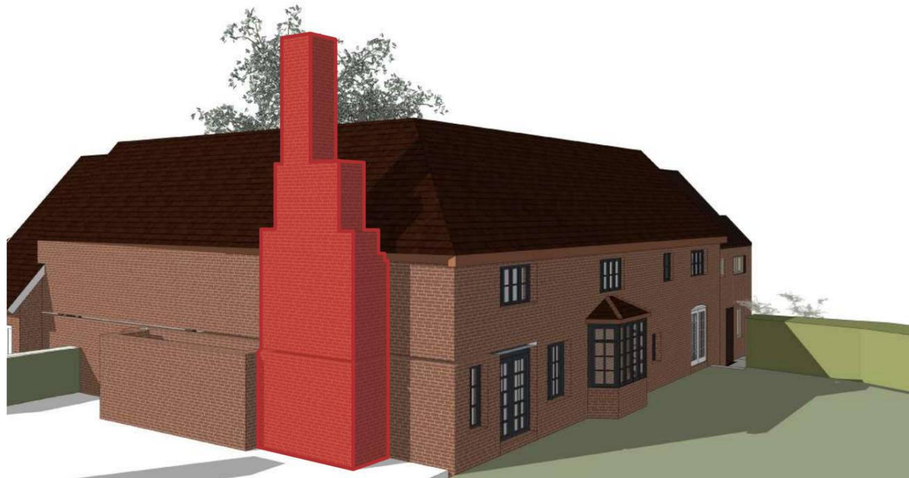
Fig.18: Existing chimney stack on north elevation - stepped and break fronted (see Fig. 22)
