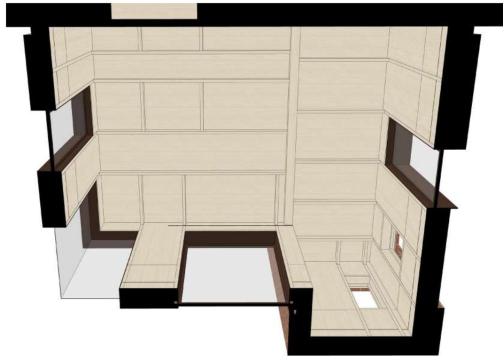
Fig.37: Asymmetrical ceiling arrangement of oak beams that junction with oak posts which align with the window frames
