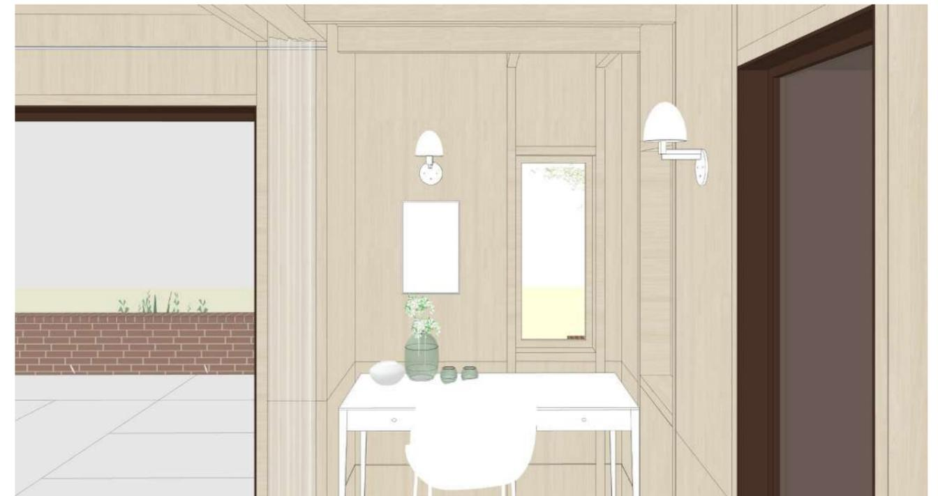
Fig.39: Oak beams line up with oak window frame posts to create oak infill panels
