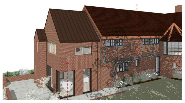
Fig.26: Brick 'panels' proposed to reference the existing post and beam brick infills
