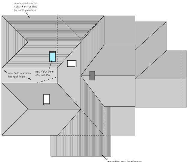
new gabled roof to extension to align with existing roof slopes
