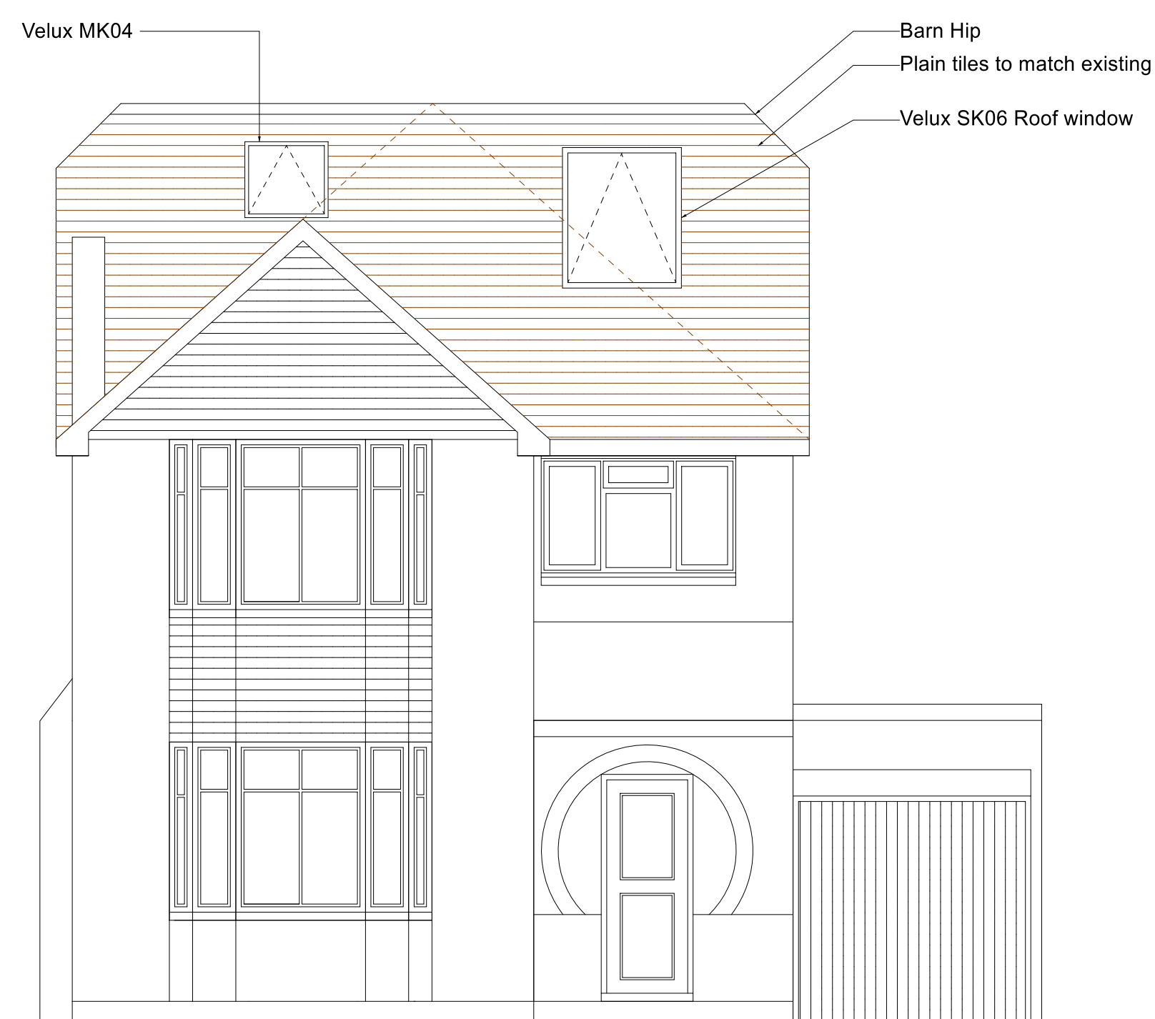
FRONT (EAST) ELEVATION
