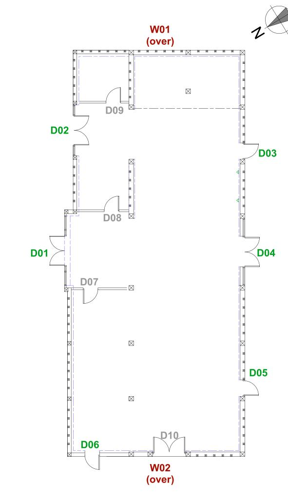
**EXTERNAL DOORS & WINDOWS** 1] EXISTING DOORS ARE FORMED OF; HARDWOOD TIMBER FRAMED SIDE HUNG PANELS/CASEMENTS, STAINED MATT BLACK WITH SINGLE GLAZED UNITS. TRADITIONAL METAL HINGES / LATCHES. TIMBER SILL AND PAINTED TIMBER WINDOW BOARDS WITH BULLNOSE PROFILE, STAINED MATT BLACK.
