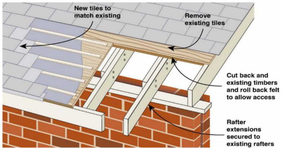
Figure 6 Eaves Roofline Extension Example
