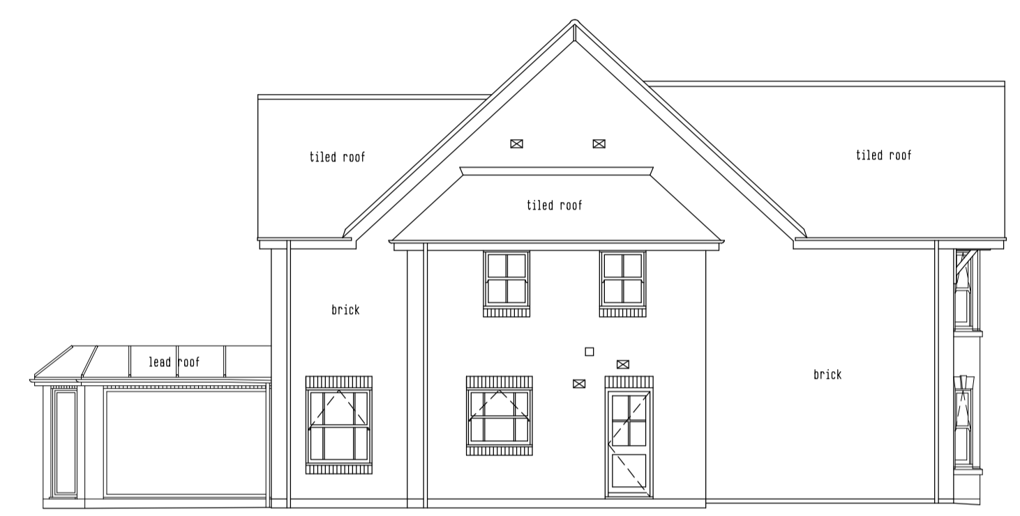
SIDE ELEVATION AS EXISTING
