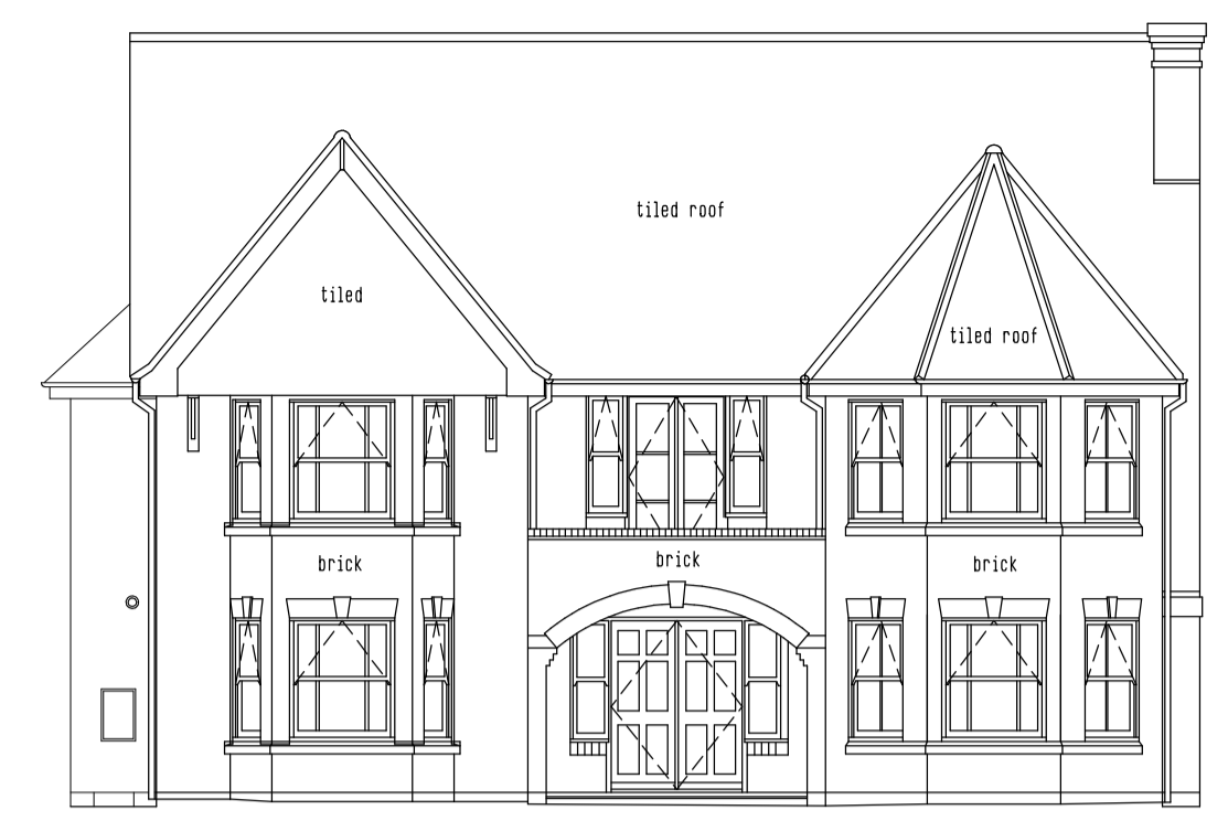
FRONT ELEVATION AS EXISTING
