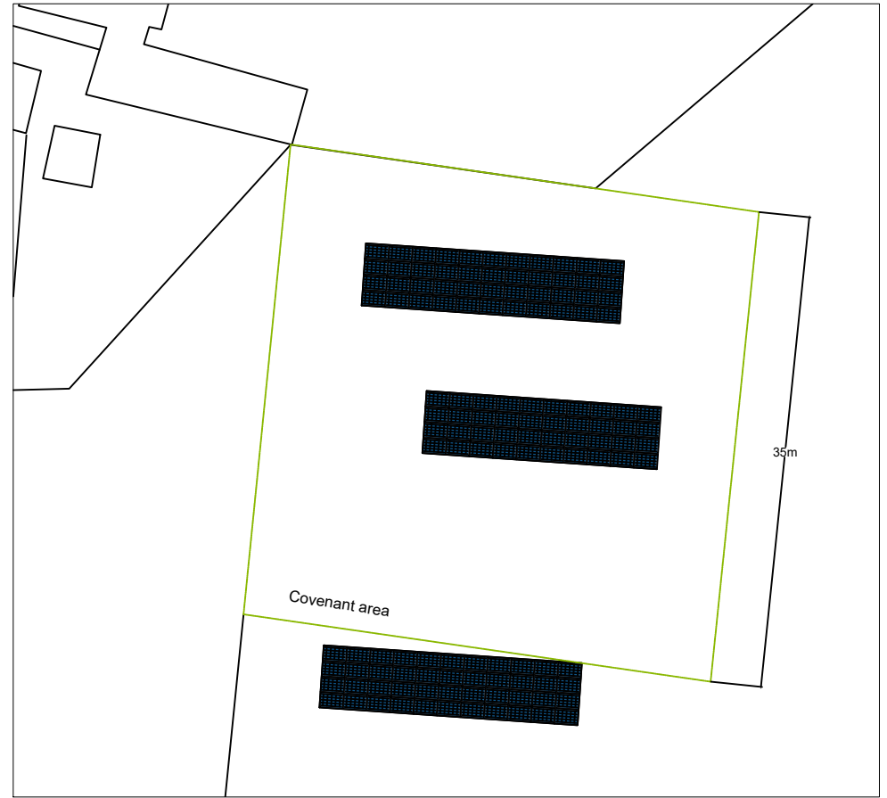
Proposed ground mount system extension comprising of 44 Canadian Solar 410w modules. New solar extension to be placed outside of existing covenant area.
