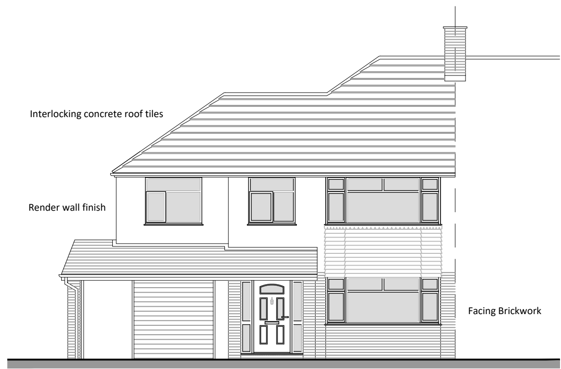
South West Elevation
