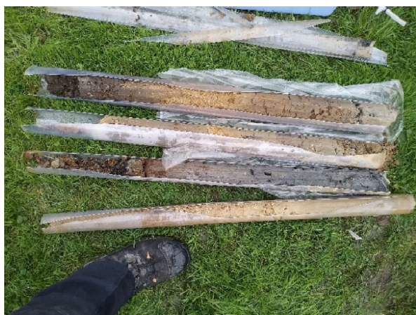
Photo 5: Recovery from WS05, showing deeper made ground onto Head Deposit and Gault Formation clay
