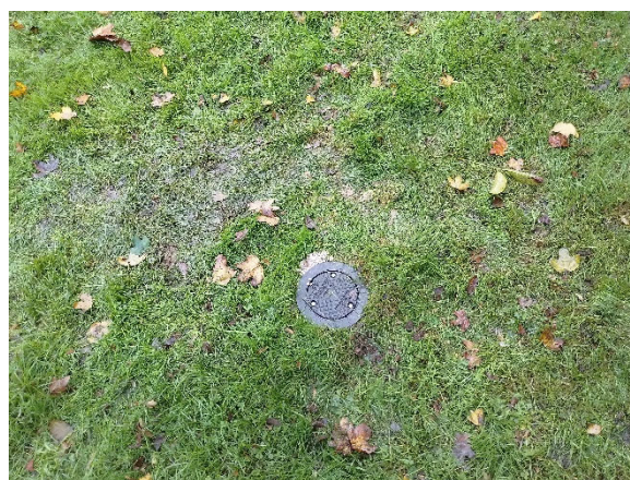
Photo 6: Installed monitoring well set flush with surface
