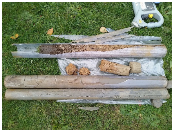
Photo 5: Recovery from WS05, showing deeper made ground onto Head Deposit and Gault Formation clay
