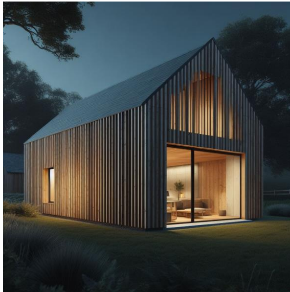
Fig 23. Concept Image with hit and miss timber cladding over windows to emphasise the barn aesthetic
