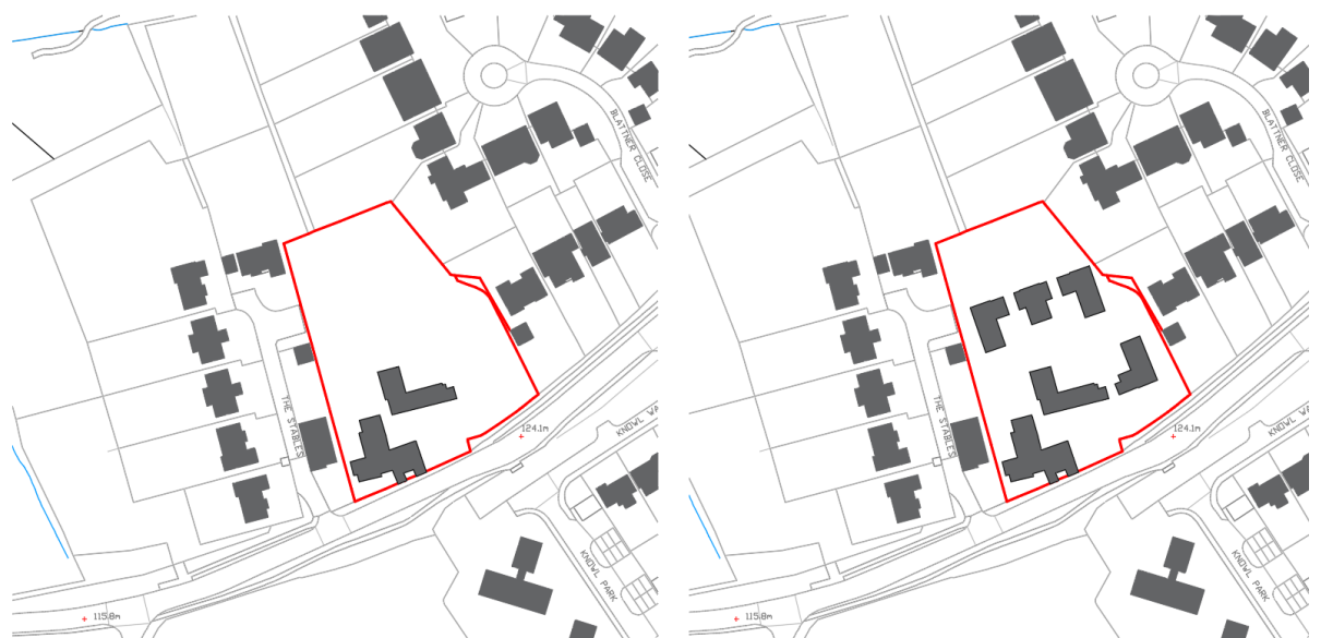
Fig 26. New buildings arranged with existing Barn and Farmhouse to form a traditional farmstead pattern
