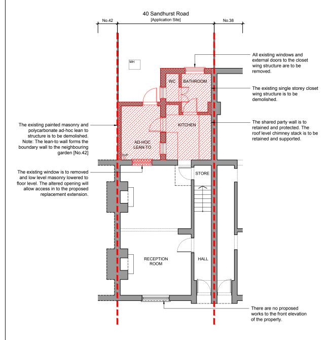
Demolition - Ground Floor Plan
