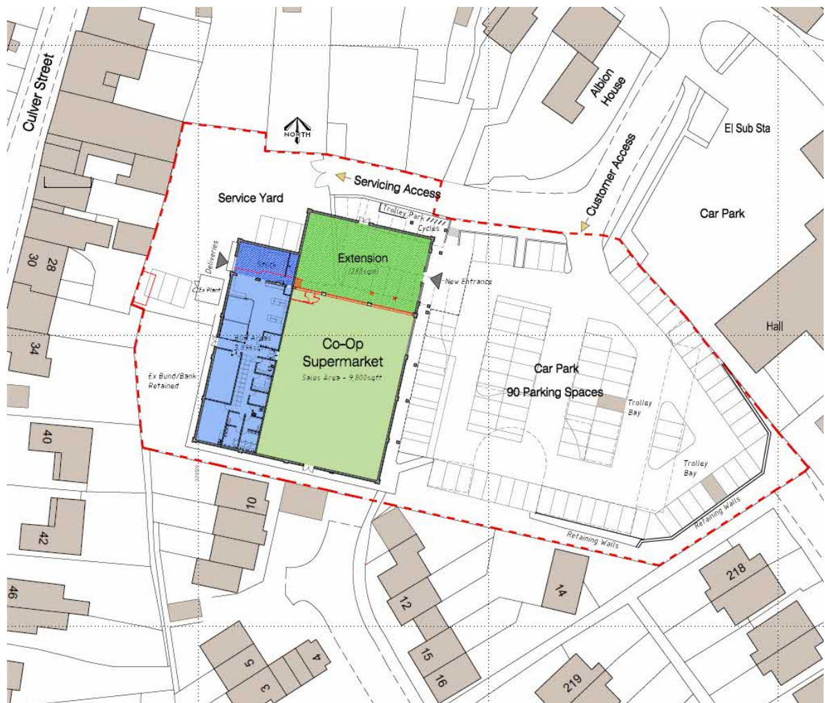
Proposed Extension Plan – extract from Gould Singleton Architects Drawing No 17-1622/300 (Not to Scale)
