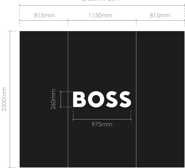
Existing cash desk back wall to be clad in 3mm matt black dibond panel, with angle capping around the edge.
