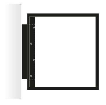
Projecting sign, internal framework clad in 2mm aluminium panels, coated RAL 9005 (Jet Black) Matt Logo to be push through, flush inlaid in opal 030 acrylic, internally illuminated via warm white LED units (5000K).
