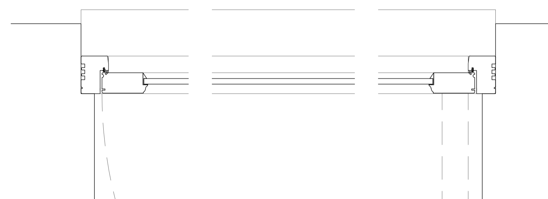
1 PROPOSED EXTERNAL DOOR TYPE 2 JAMB C303 scale 1:5
