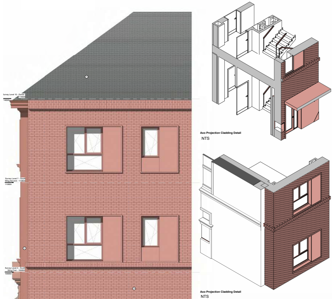
Proposed brick string coursing on courtyard facade to Police Wing to reference detail on adjacent historic façades.
