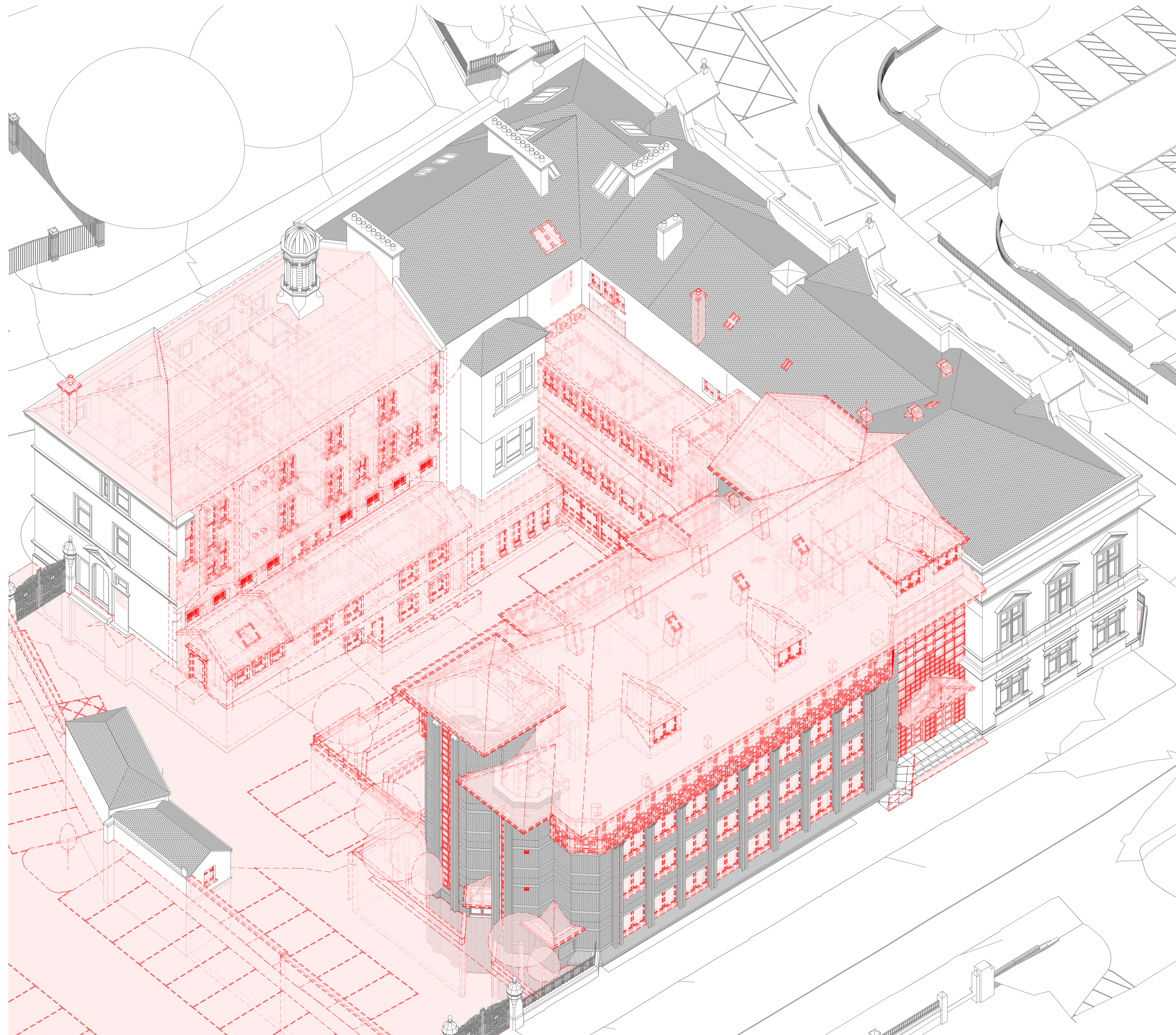
Existing Axo South _Demolition
