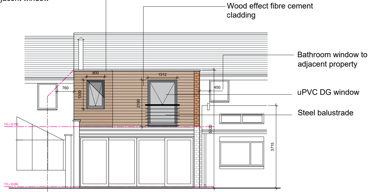
South West Elevation
