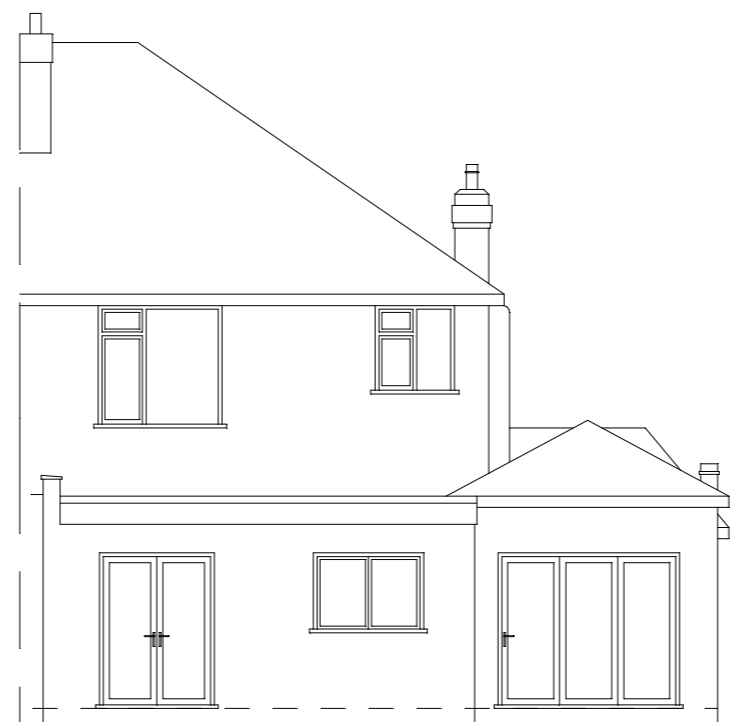
EXISTING REAR ELEVATION
