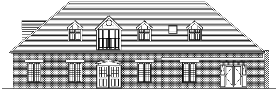
Proposed East Elevation of West Building Scale 1:200
