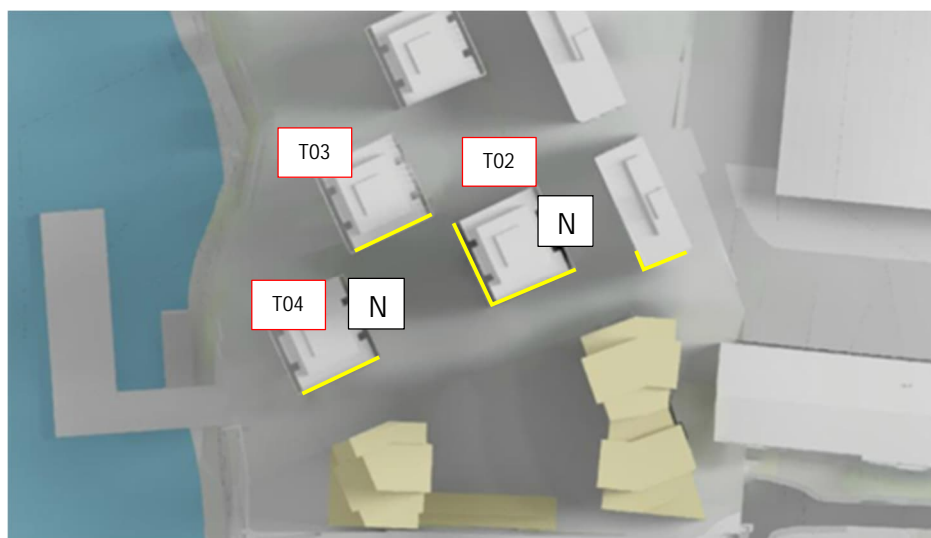
Fig. 28 – North orientated facades on the assessed blocks of Morden Wharf & elevations (yellow) assessed for sunlight impact
