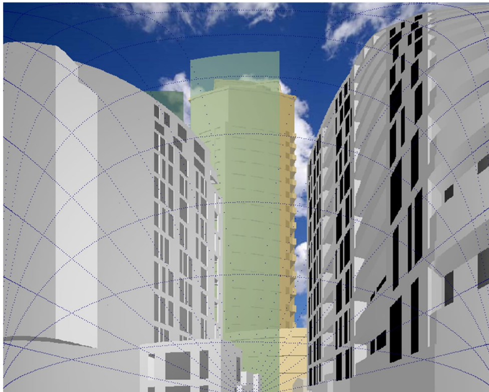
Fig. 27 – Waldram diagram of Trefoil House 'Ground W4' (extant mass in green & Applicant's proposal is shown in yellow [Telcon tower])
