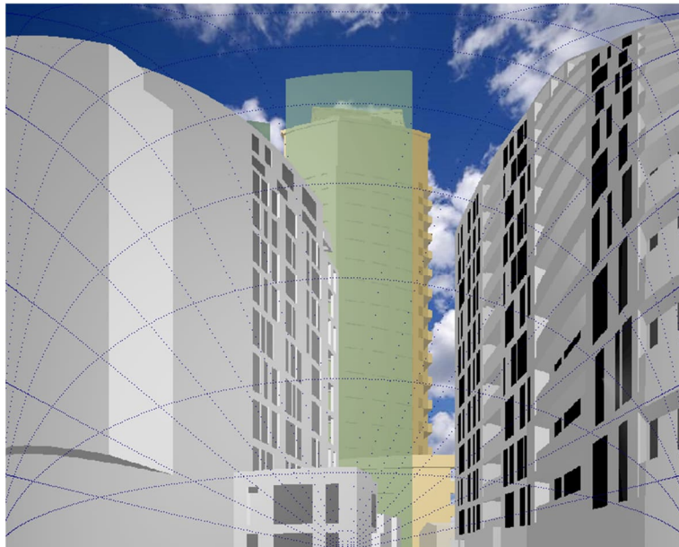
Figure 11 – Trefoil House Waldram diagram (Ground 'W5') looking towards Telcon tower on the Applicant site
