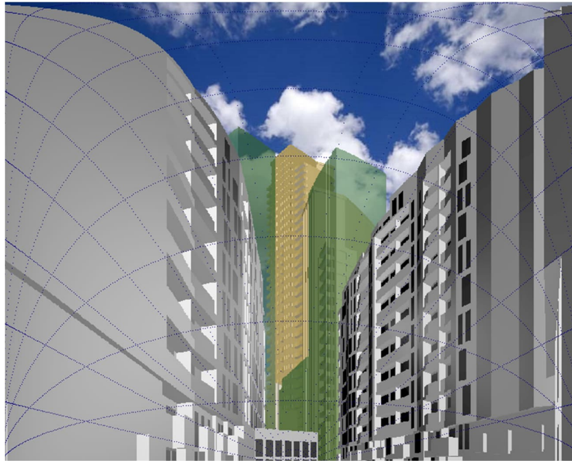
Figure 16 – Waldram diagram for Lariat Apartments (Ground W4) showing the extant scheme (green) and the Applicant's proposal (yellow [Telcon tower]) between Distel Apartments & Bowline Court
