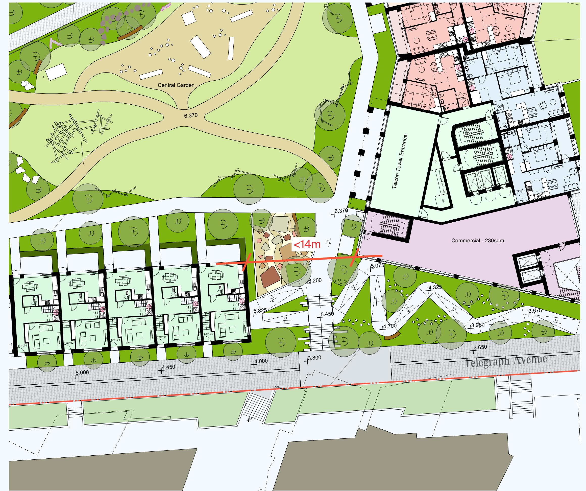
PROPOSED PODIUM LEVEL PLAN WITH TELEGRAPH BLOCK UNITS REMOVED TO INCREASE ENTRANCE SPACE AND REDUCE WIND ACCELERATION
