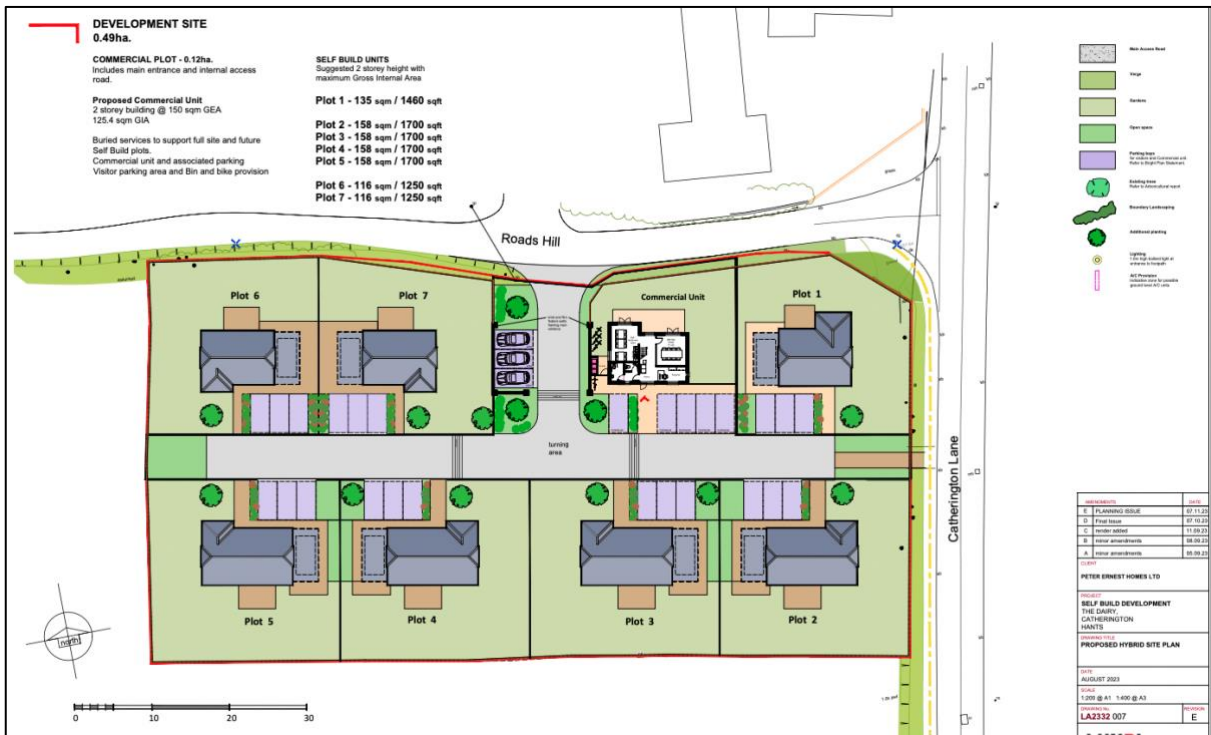
Figure 2. A proposed plan showing the hybrid application with the detailed layout of the commercial unit and illustrative drawings of the residential plots. Provided by Lundi Architects. Dated August 2023. Drawing no. LA2332 007 Rev E.
