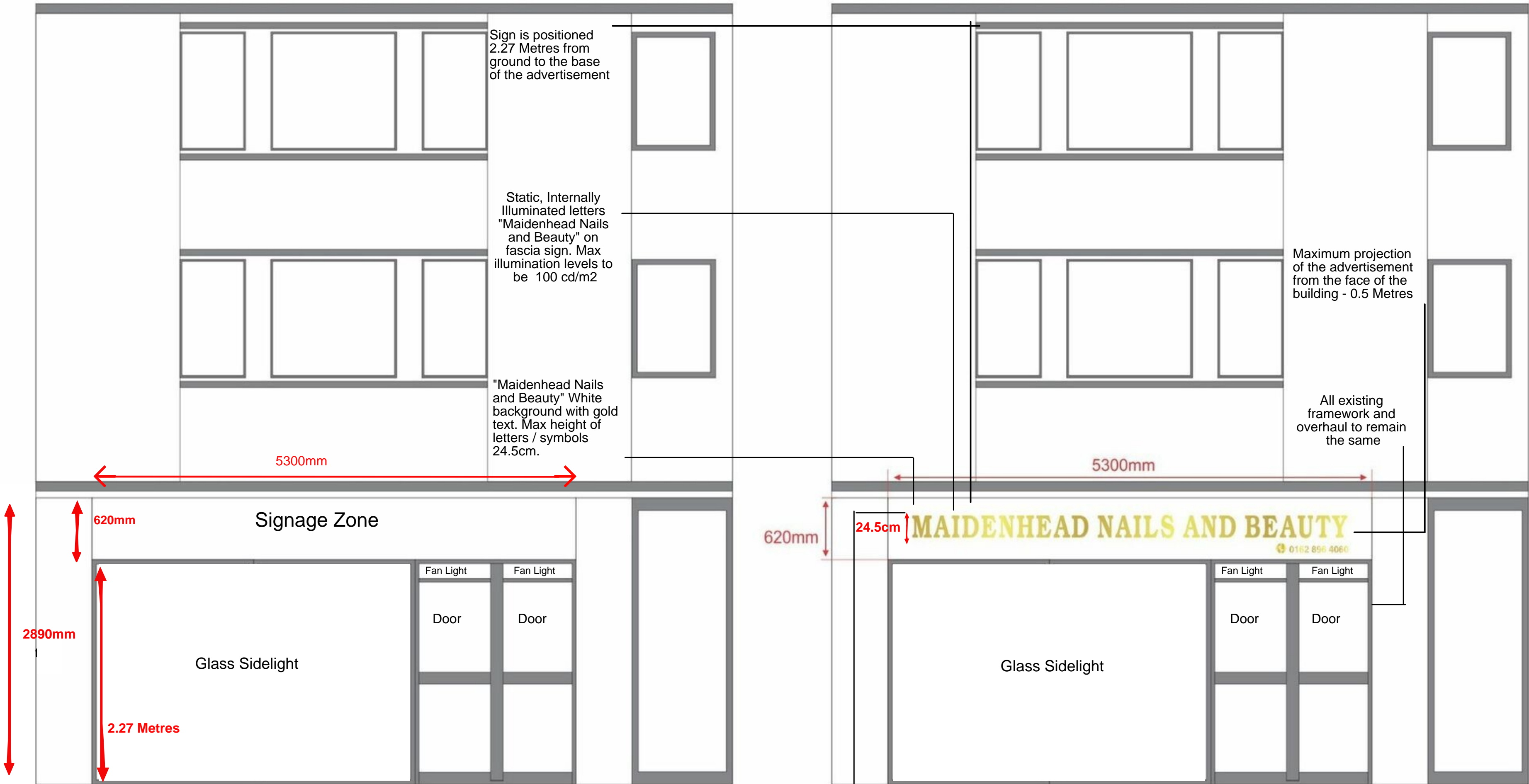
Aluminium Composite Fascia Sign. Height: 0.62 metres Width: 5.3 metres Depth: 0.03 metres
