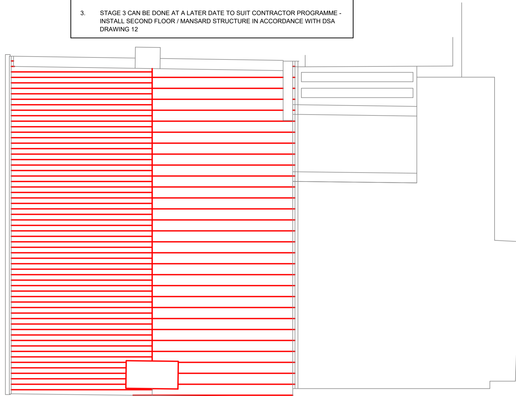
ROOF PLAN SHOWING DEMOLITION (PHASE 1, STAGE 1) 1:50
