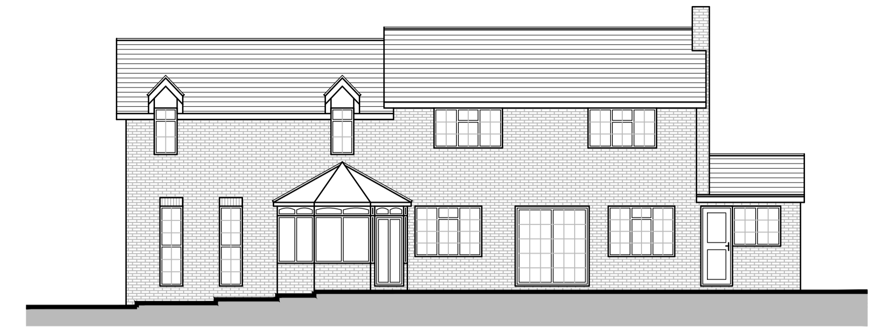
EXISTING REAR ELEVATION 1:100
