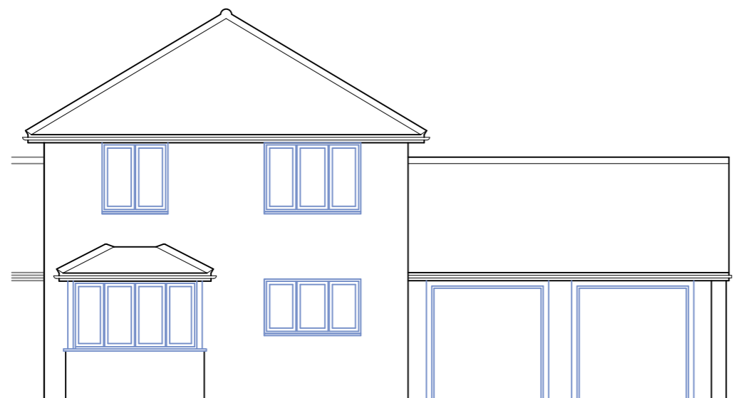
EXISTING FRONT ELEVATION
