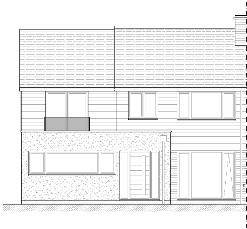
Front (north-facing) Elevation 1:100
