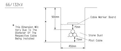
Note:- Pilot Cable Should Be Laid For 50% Of The Total Route Length On The Right Hand Side Of The Circuit & For The Remaing 50% On The Left Hand Side Of The Circuit
