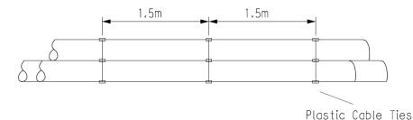
33,66 & 132kV Cables Laid In Trefoil & Cable Tied At 1.5m Intervals (1m At Bends)
