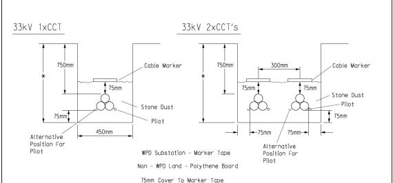
75mm 3mm To Dust, Limestone Or Granite Fine Stone Dust Bedding & Blinding
