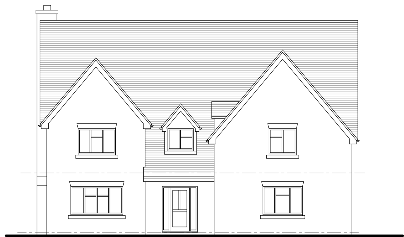
FRONT EXISTING ELEVATIONS 1:100
