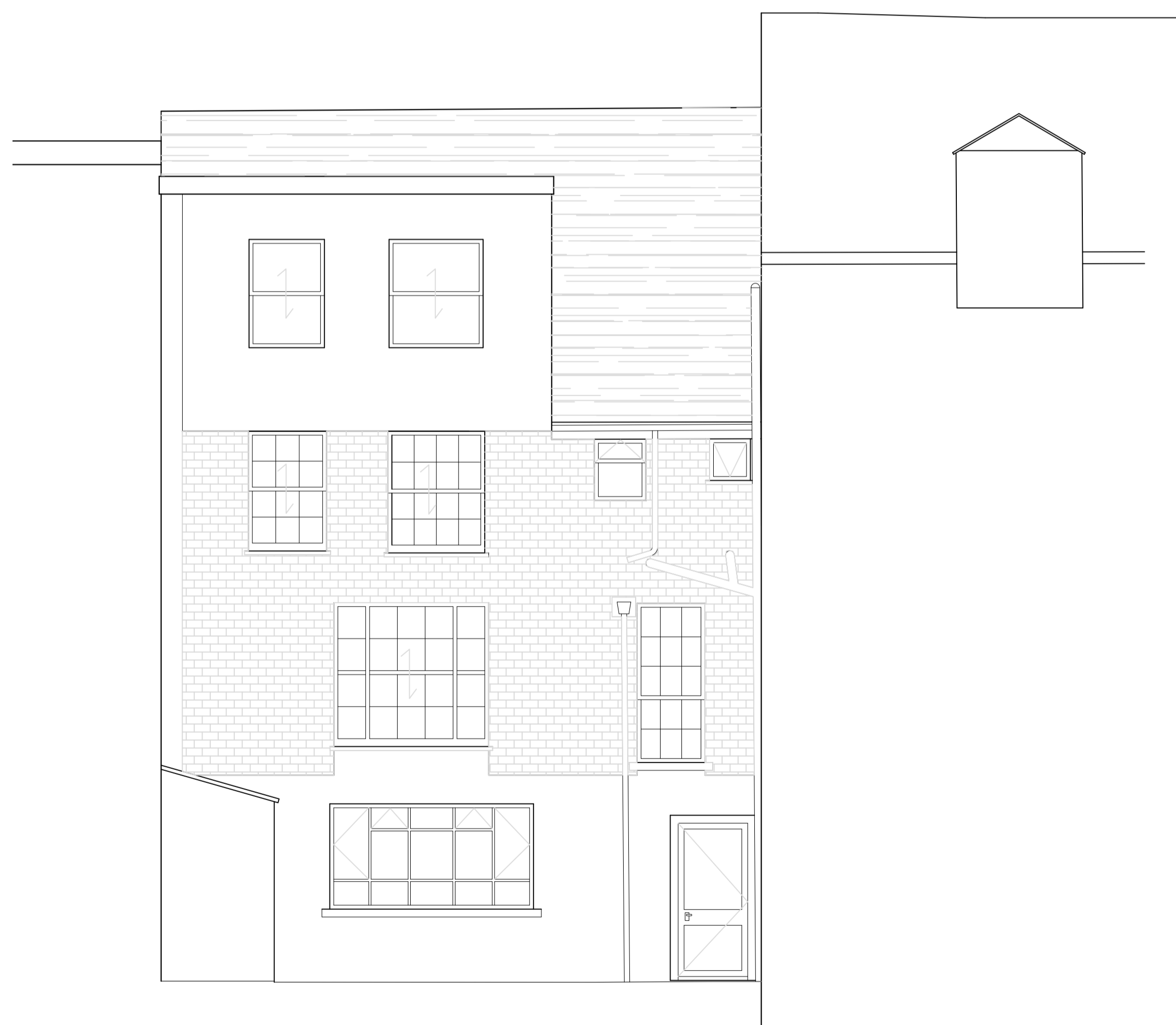
EXISTING REAR (SOUTH WEST) ELEVATION 1:50
