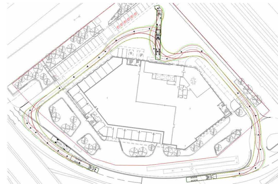
Figure 5 Swept Path Analysis (16.5m Articulated Vehicle)
