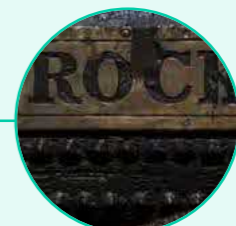
LASERCUT ENGRAVED AND FILLED LETTERING
