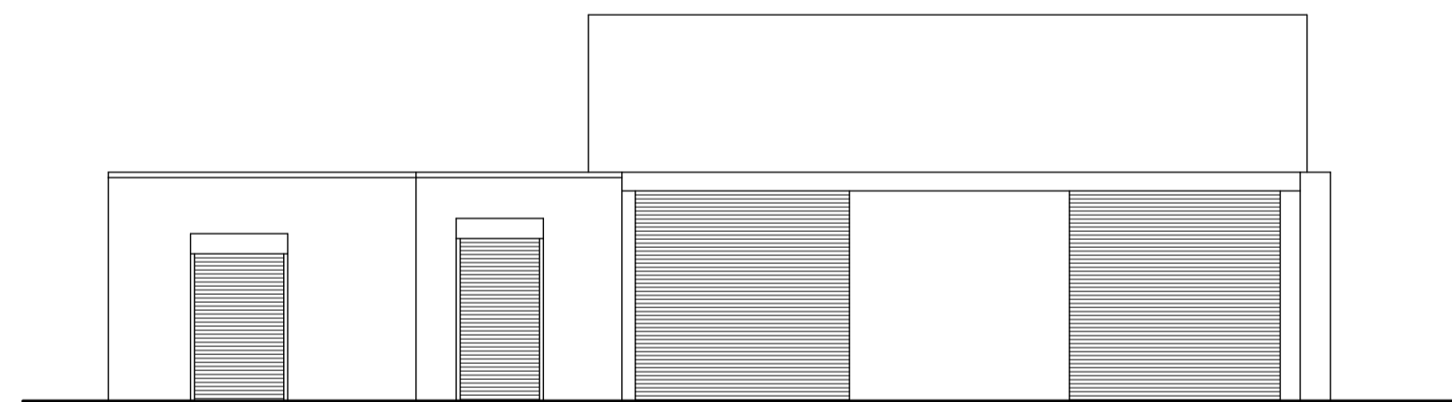
Workshop Building - South Elevation Scale 1:100
