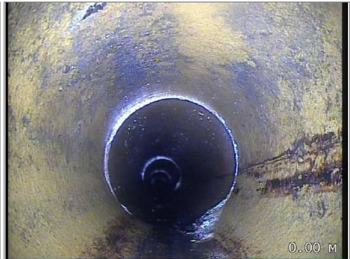
Water level 0% height/diameter
