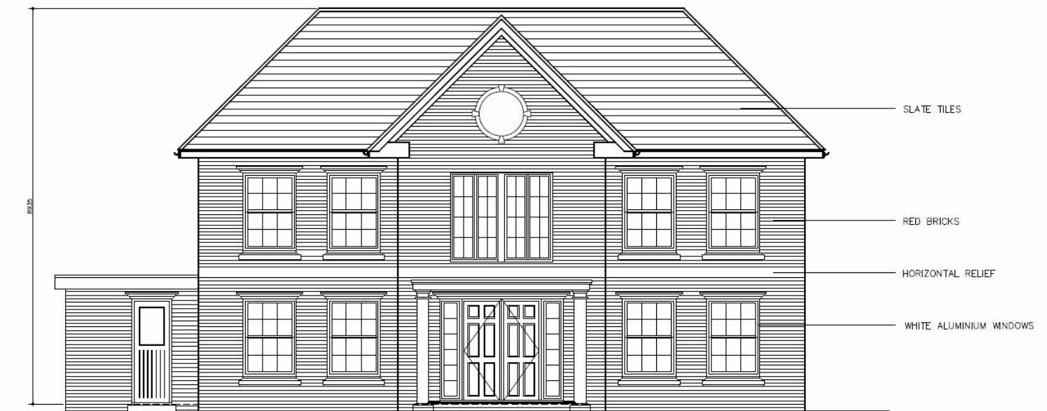
FRONT ELEVATION – NORTH
