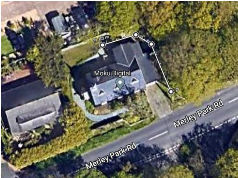
Figure 1 - Aerial plan indicating proposed 21m length and alignment of barrier
