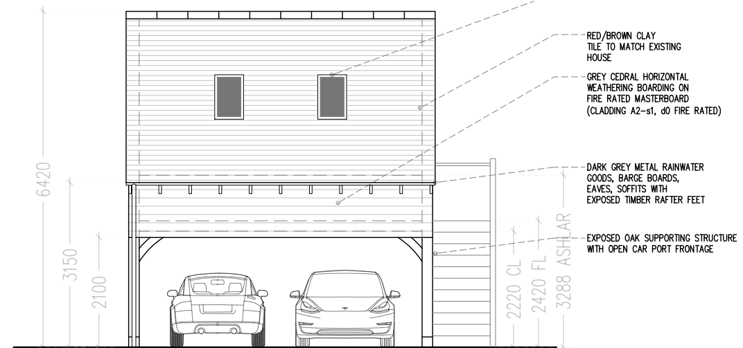
PROPOSED SOUTH EAST ELEVATION (SEAFIELD ROAD ELEVATION)
