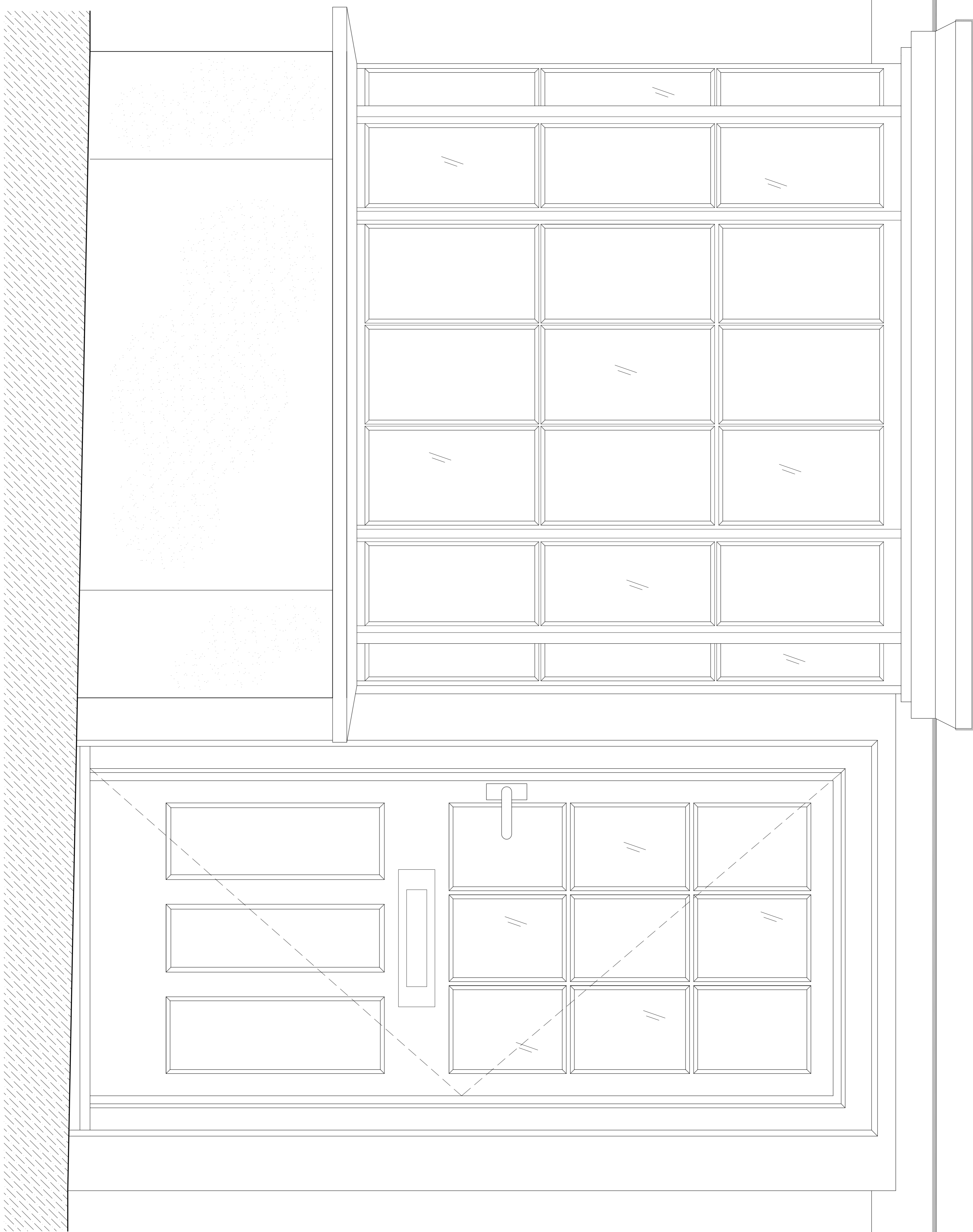
Proposed bay window and door elevation SCALE: 1:5
