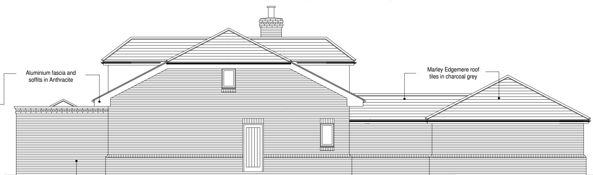
PROPOSED SOUTH ELEVATION ( scale 1:100@A3 )
