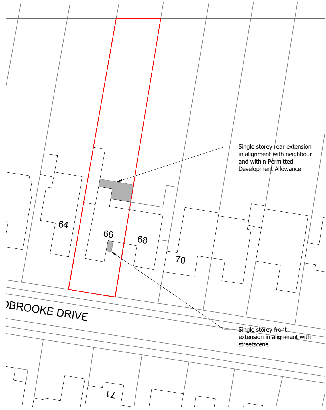
01 Proposed Block Plan Scale 1:500
