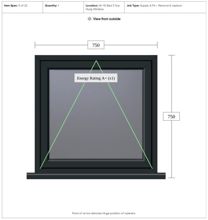
Frame:Short Leg SquareSash:Flush BevelBead:BevelCill:155mmFrame Joint Type:MitredSash Joint Type:Mitred
