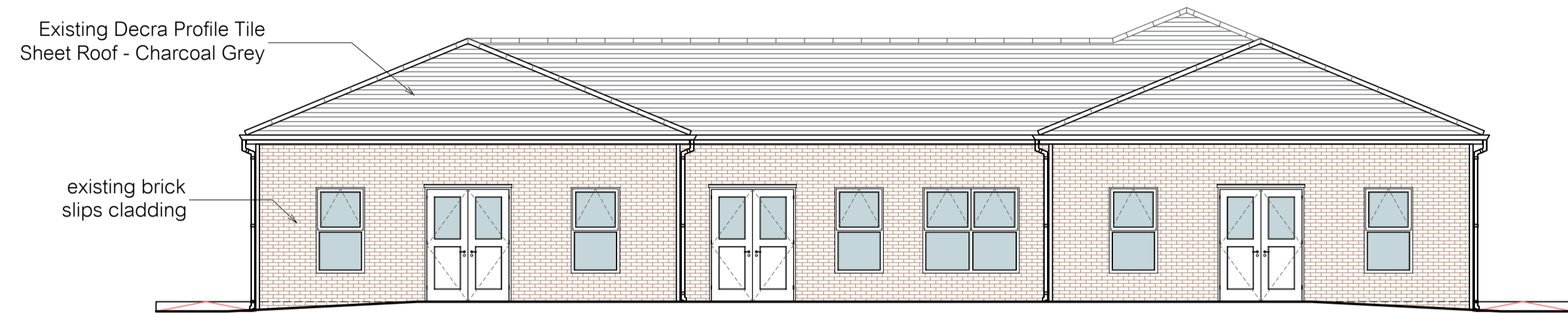
Existing Northeast Elevation
