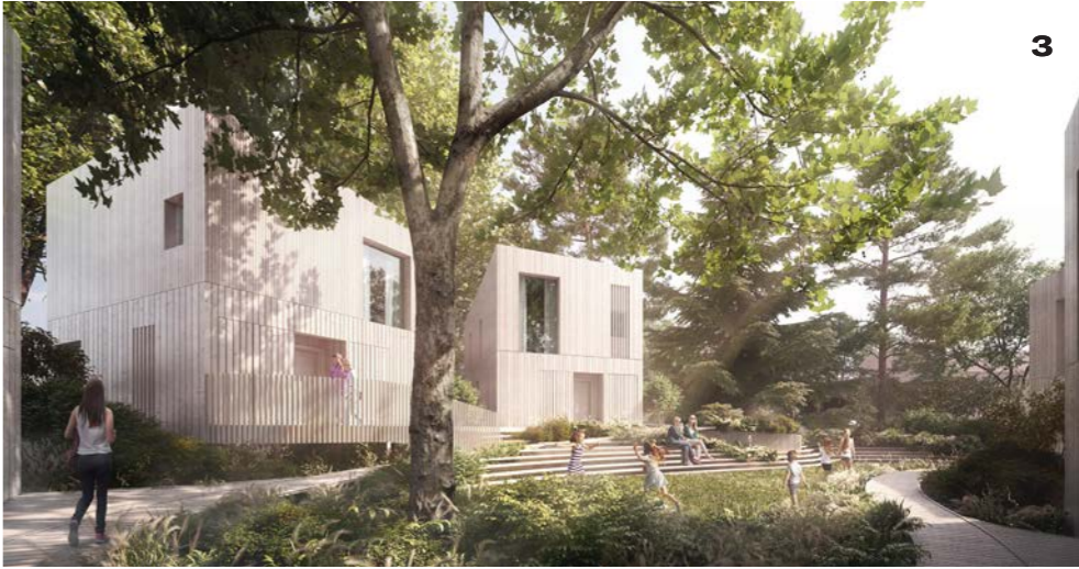
3 Honor Oak Park: Sensitive approach to all existing tree protection orders and root protection areas across the site to provide 6 cabin style houses built out of lightweight timber construction on a raised deck to protect the tree roots
