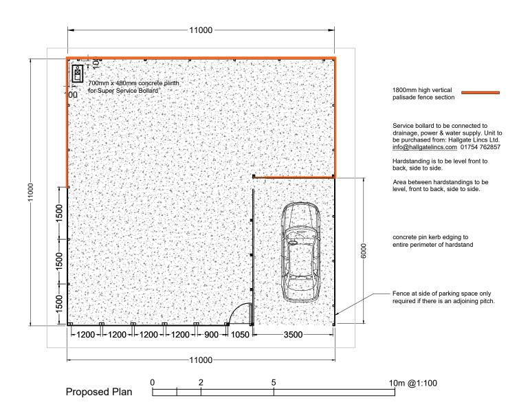
Fencing: Vertical timber palisade sections 100mm x 25mm with 25mm spacing, fixed to 47mm x 125mm cant rail, bolted to 100mm x 100mm timber post, pressure treated with clear preservative and angled top.
