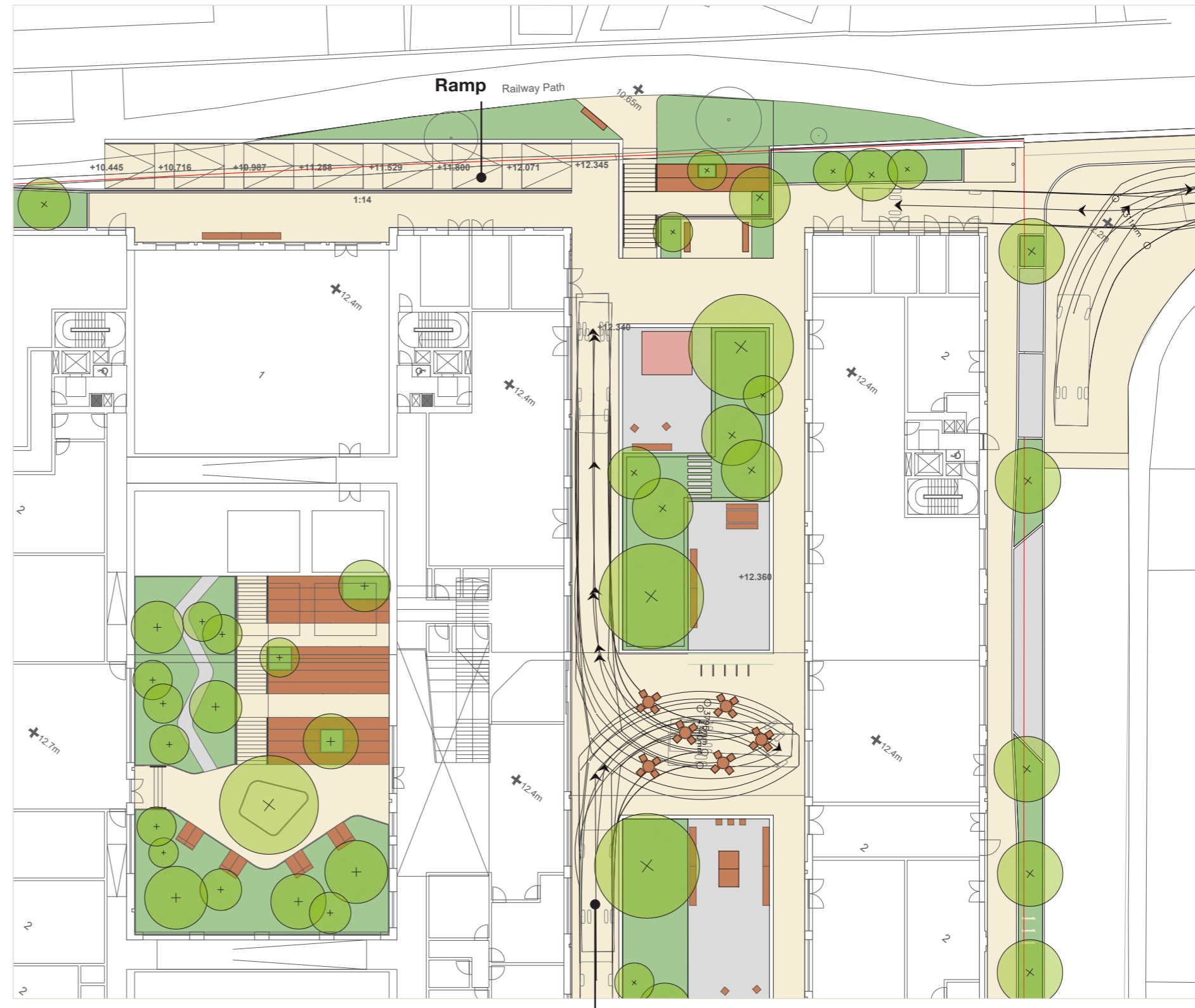
Fire tender/ maintenance vehicle tracking
