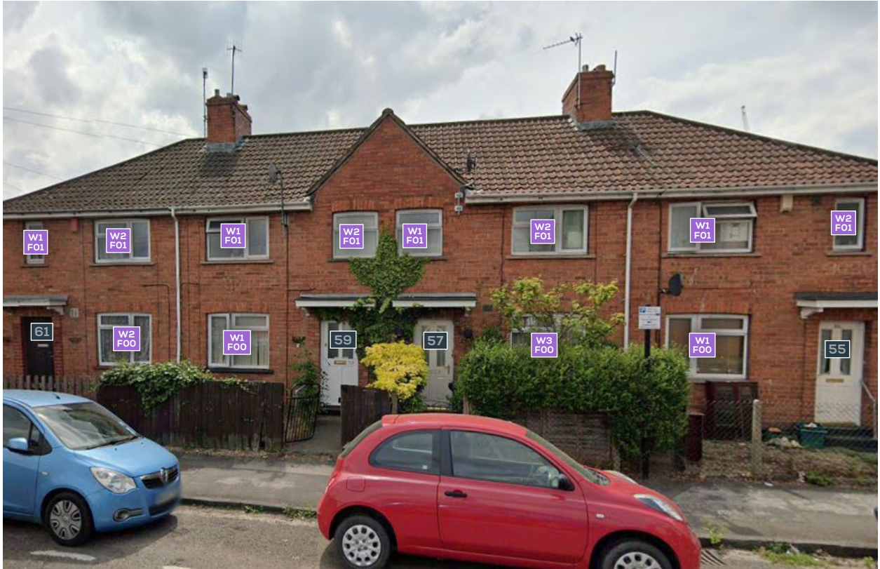
Figure 04: Window Map highlighting those windows which do not meet the BRE's recommendations for VSC (purple).
